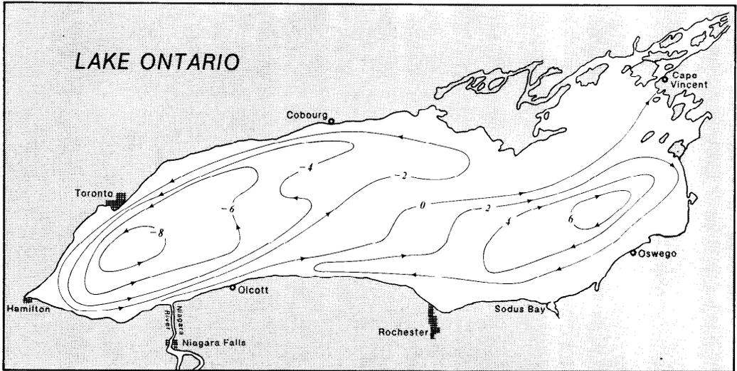
Fig. 2. Steady state model transport lines ( $10^{10} \text{ cm}^3 \text{ s}^{-1}$ ) in Lake Ontario for  $5 \text{ m s}^{-1}$  northeast wind.
