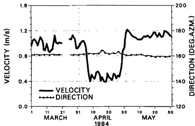
FIG. 7.—St. Clair River Current Meter Velocity and Direction, March–May, 1984
