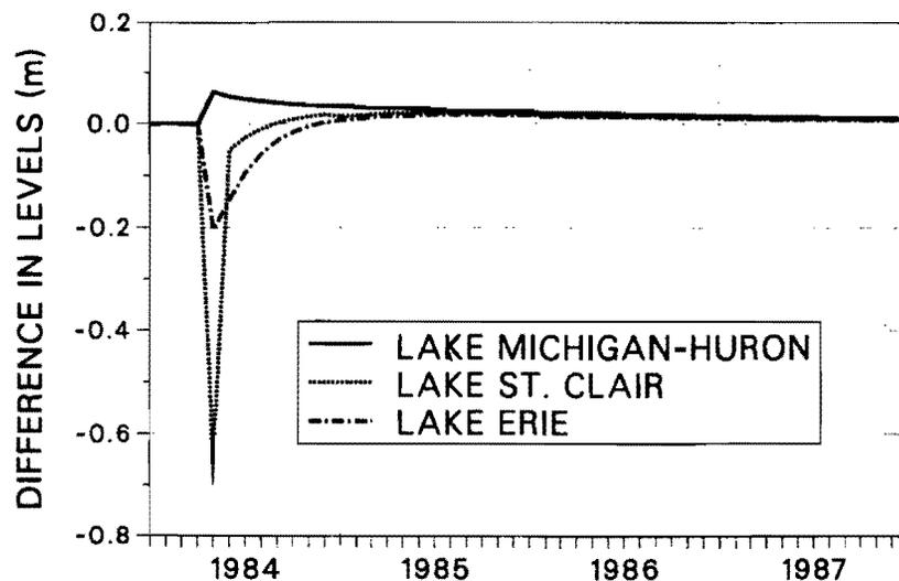
FIG. 8.—Effect of Ice Jam on B-O-M Levels, 1984–87
