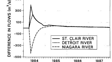
FIG. 9.-Effect of Ice Jam on Flows, 1984-87
