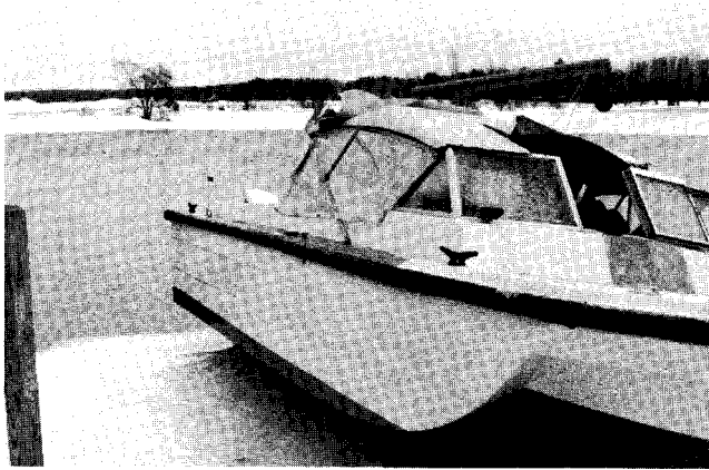
FIG. 3. The boat immediately after completion of the pre-ice cruise. Note extensive icing on the windshield.
