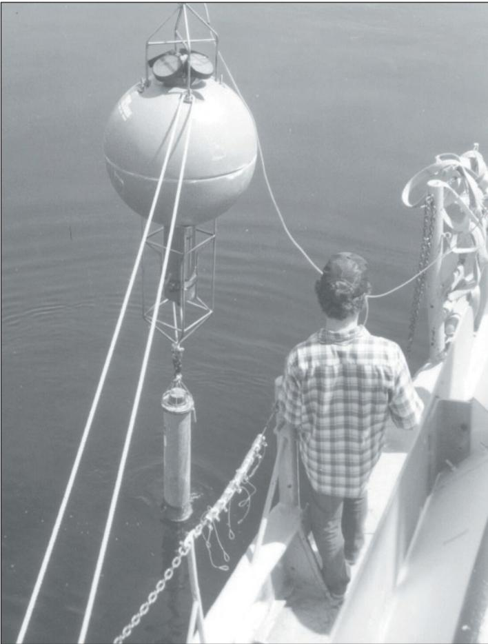
*Installation of current meter in the Straits of Mackinac from the NOAA Research Vessel Shenehon. The current meter is placed inside a spherical flotation collar above an acoustic release device and anchor.*
