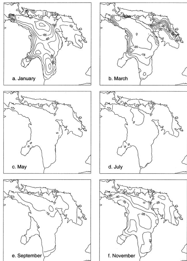
**FIG. 4.** As in Figure 3, but for sensible heat flux, and with a contour interval of  $5 W/m^2$ .
