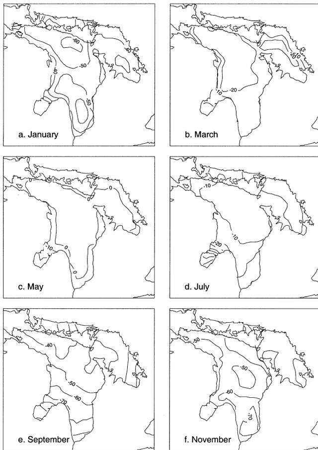
**FIG. 3.** The spatial distribution of 1992 to 1995 monthly mean latent heat flux ( $W/m^2$ ) over Lake Huron during the month of (a) January, (b) March, (c) May, (d) July, (e) September, and (f) November. The contour interval is  $10 W/m^2$ .
