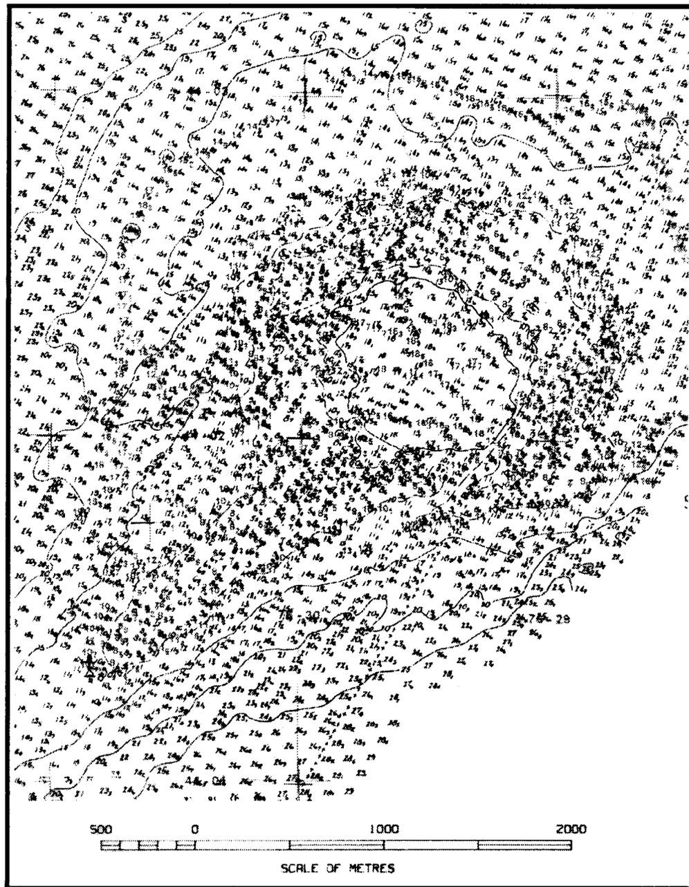
*FIG. 2. Sounding data coverage for the Charity Shoal area, illustrating the distribution of data employed in construction of the detailed bathymetry. Spot depths are in meters and tenths. Both U. S. and Canadian bathymetric soundings are shown. Five-meter contours delineate the basic features of Charity Shoal and adjacent topography.*
