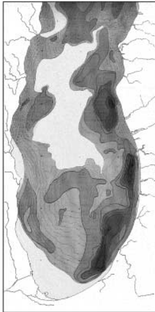
Fig. 6. Sediment deposition thickness in Lake Michigan (after Foster and Colman, 1992). The five ranges of sediment thickness depicted in the map are (from lightest to darkest): 1–2 m, 2–6 m, 6–10 m, 10–14 m, and > 14 m.
