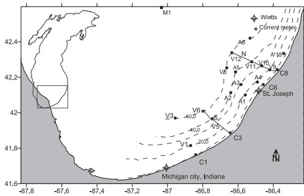
**Figure 1.** Geometry and bathymetry of southern Lake Michigan showing meteorological and current meter stations (A: ADCP; V: VACM, C: SACM).
