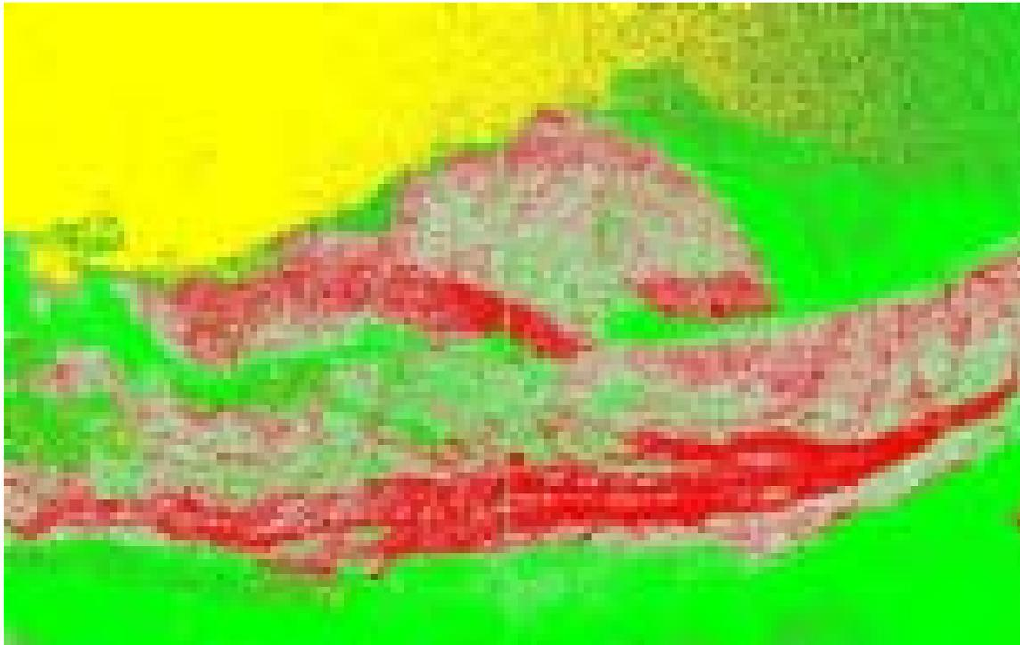
**Figure 7:** Ice classification results in Whitefish Bay (corresponding to the brash ice area in Figure 4): Red for brash ice, green for patchy snow on snow ice over lake ice and consolidated ice floes, and yellow for black ice with thin snow cover.
