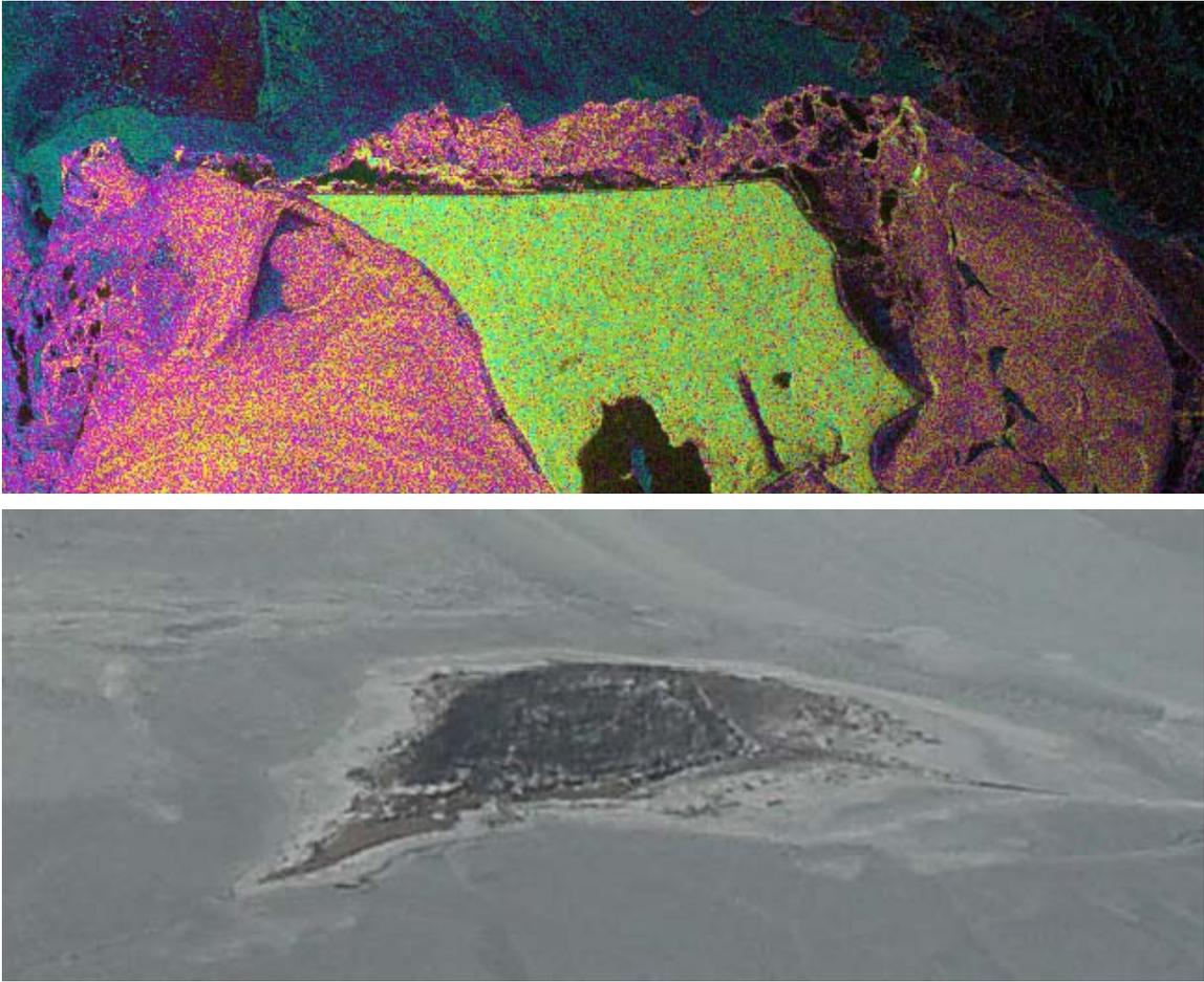
**Figure 8:** Images of ice surrounding Chambers Island in Green Bay, Lake Michigan: (a) Top panel is an L-band AIRSAR image for an ice area in Green Bay with color proportional to the ratio of the HH and VV polarimetric channels, and (b) bottom panel is an aerial photograph of the same location. Note that the look angles and azimuth orientations are different between the two images.
