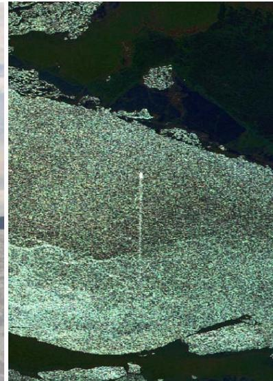
**Figure 6:** Mackinaw in SAR image with trailing ship track
