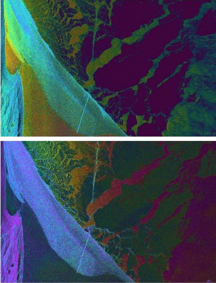
**Figure 9:** Thunder Bay image for combination of HH, VV, and total radar brightness at C band (top panel) and L band (bottom panel).
