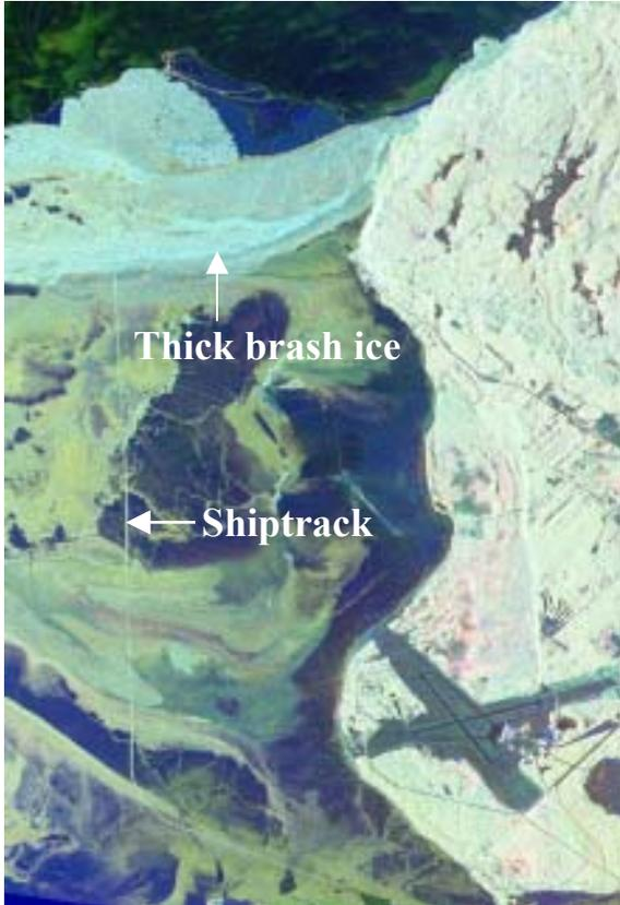
**Figure 4:** Zoomed-in SAR image revealing the US Coast Guard Mackinaw ship track encountering thick brash ice in the Whitefish Bay.
