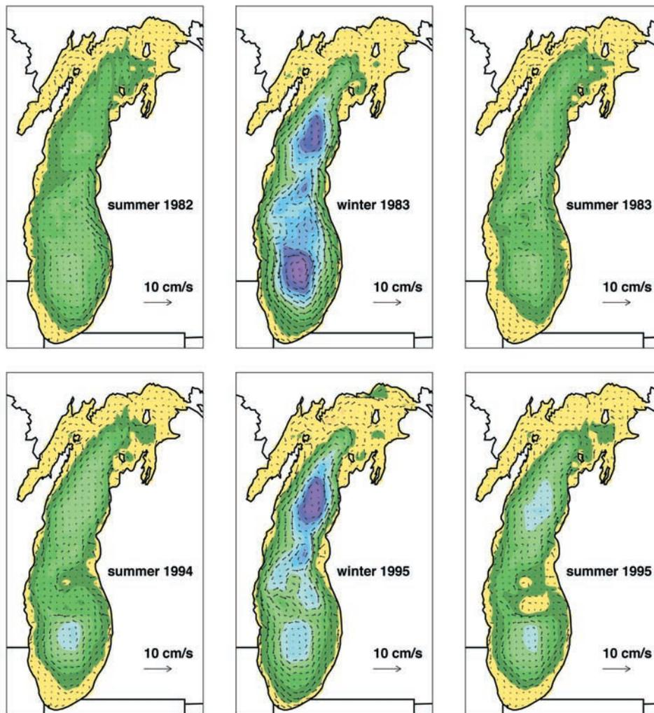
**Figure 1.** Seasonally averaged Lake Michigan currents from 1982 to 1983 and 1994 to 1995 numerical model simulations by *Beletsky and Schwab* [2001]. Summer is May–October, and winter is November–April. Colored shading represents stream function values. Yellow is positive (generally anticyclonic vorticity), and the green-blue-purple areas are negative stream function (generally cyclonic vorticity).
