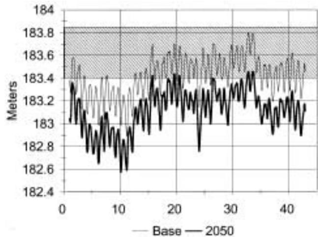
**FIG. 9.** Lake Superior levels based on Canadian Climate Centre model, CGCM1. The comparison of Base (1961 to 1990) with 2050 (2030 to 2071) indicates a drop in lake levels of approximately 0.3 meters due to greatly increased evaporation caused by warmer air temperatures.
