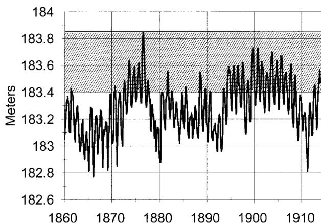
**FIG. 2.** 1860 to 1913 Lake Superior hydrograph. The hatched area shows regulation limits established by the 1914 Order of Approval, 183.4 and 183.86 m, IGLD 85.
