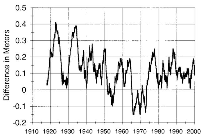
**FIG. 5.** The difference between recorded and simulated “pre-regulation” levels for Lake Superior. Positive values indicate that regulated levels on Lake Superior are higher than they would have been under “natural” conditions, often by 15 to 20 cm.
