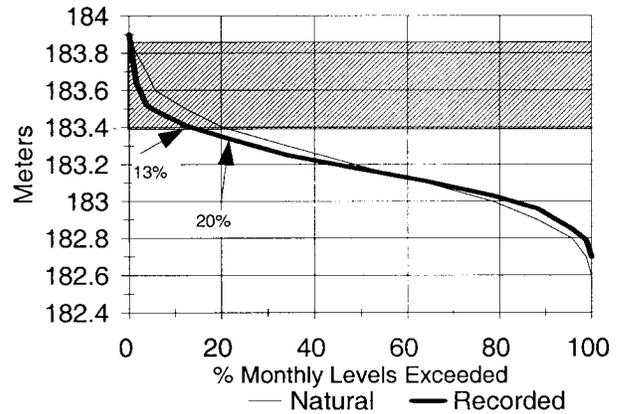
**FIG. 7B.** Frequency distribution for 1921 to 1972; regulation based on Superior only. When regulation was based on Superior levels only, high levels were reduced by 7%.
