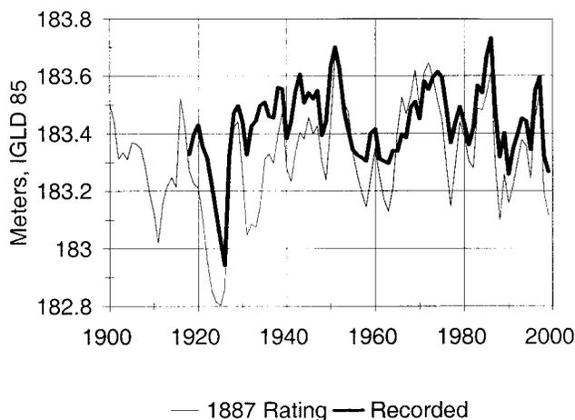
**FIG. 11.** Comparison of recorded levels with “natural” (1887 Rating) levels for Lake Superior. Regulation appears to have prevented (by at least 10 cm) even lower levels in the 1920s and 1960s. This also shows that regulation increased the peak high levels in the 1980s by over 10 cm.
