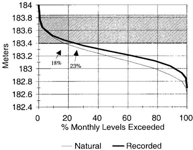
**FIG. 7A.** Frequency distribution for 1921 to 1999, the entire period of regulation. Regulation of Lake Superior has increased the occurrence of high lake levels by 5%.
