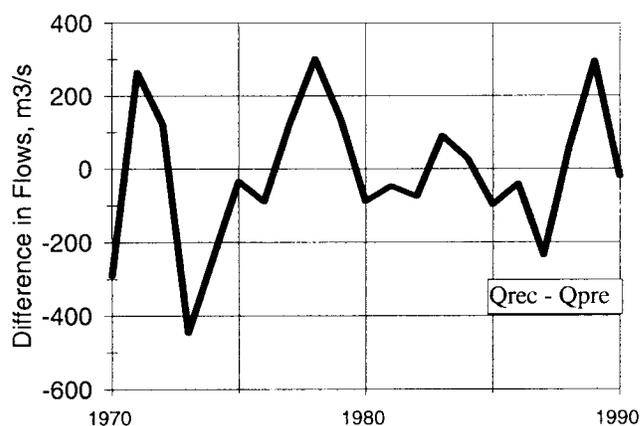
**FIG. 6.** The difference in outflows (recorded minus pre-regulation) between recorded and simulated “pre-regulation” levels for Lake Superior from 1970 to 1990. Positive values indicate that more water is being released from the lake than the “natural” condition. The negative values in the 1970s and 1980s show that water was being held on Lake Superior during these periods of high supplies.
