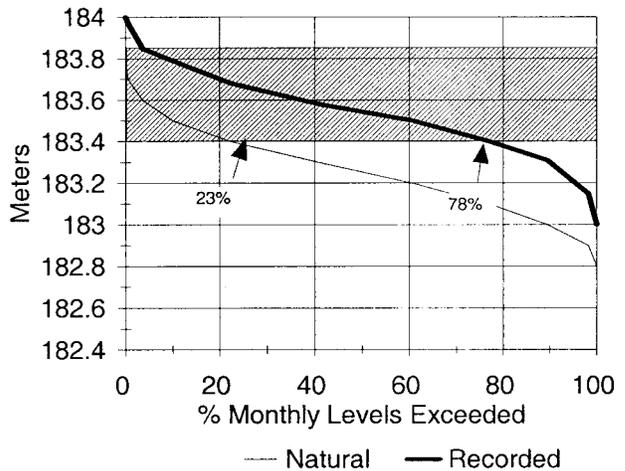
**FIG. 7C.** Frequency distribution for 1973 to 1999, regulation based on balancing. During recent years when regulation of Lake Superior was based on balancing storage between Superior and Michigan-Huron, regulation more than tripled the occurrence of high levels on Lake Superior. This period also included some very high supplies.
