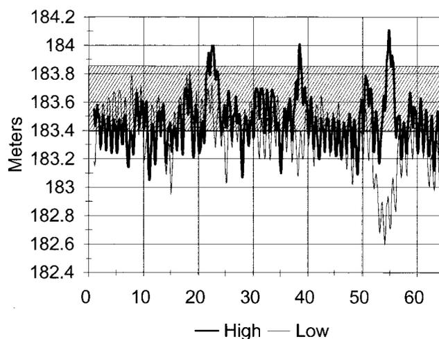
**FIG. 10.** Lake Superior levels produced by stochastically-generated series of net basin supplies. The experimental net basin supplies were developed based on present climate to provide extreme highs and lows for testing future models. This shows the levels produced by the segment with the highest supplies and the one with the lowest supplies.
