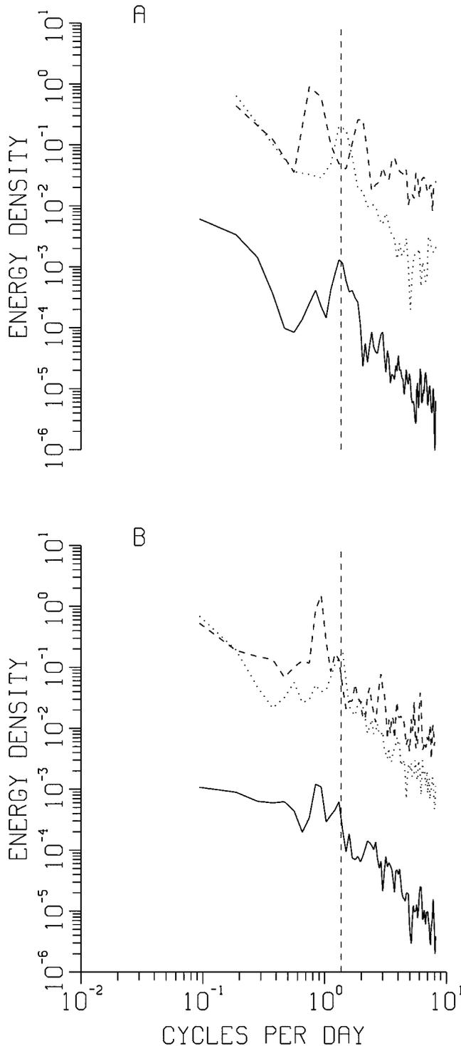
**FIG. 4.** Power spectra of the parameters during the summer deployments. The solid lines are the power spectra for the optical attenuation, the dashed lines are the power spectra for the acoustic backscatter intensity, and the dotted lines are the power spectra for the bottom current velocity. The dashed vertical lines indicate the inertial period (17.6 h) of the lake. A. Data from 1998. B. Data from 2002.
