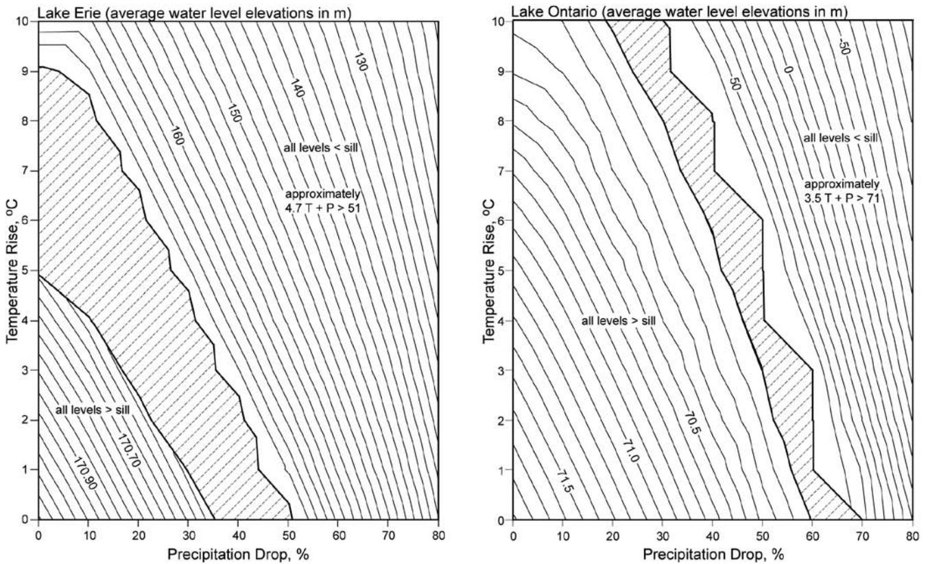
FIG. 8. Steady state lower Great Lakes average water levels as a function of temperature rise and precipitation drop relative to the present base climate.
