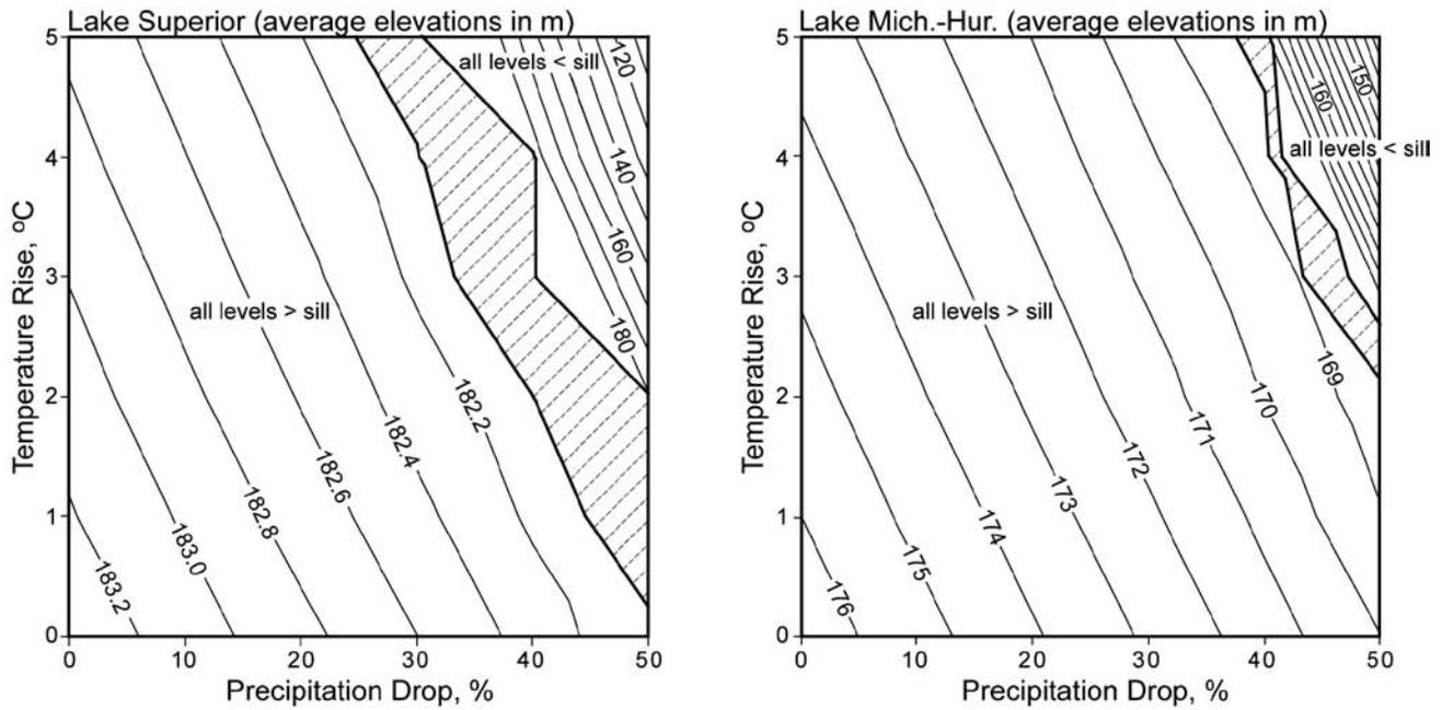
FIG. 7. Steady-state upper Great Lakes average water levels as a function of temperature rise and precipitation drop relative to the present base climate.
