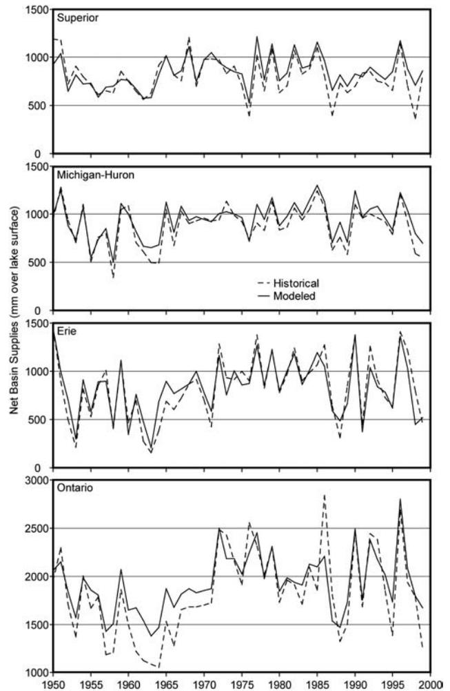
**FIG. 5. Net basin supply comparison for 1948-1999 showing reasonable agreement between water supplies based on computation of observed lake levels and flows (historical) and supplies simulated from observed meteorology (modeled).**
