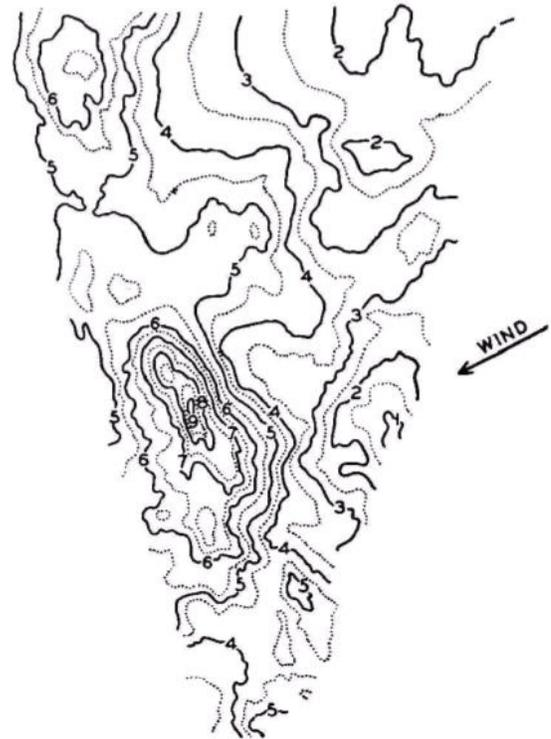
Figure 2. From Sverdrup *et al.* (1942). Topography of the sea surface derived from stereophotogrammetric pictures of the sea surface taken onboard the Meteor on January 23, 1926.
