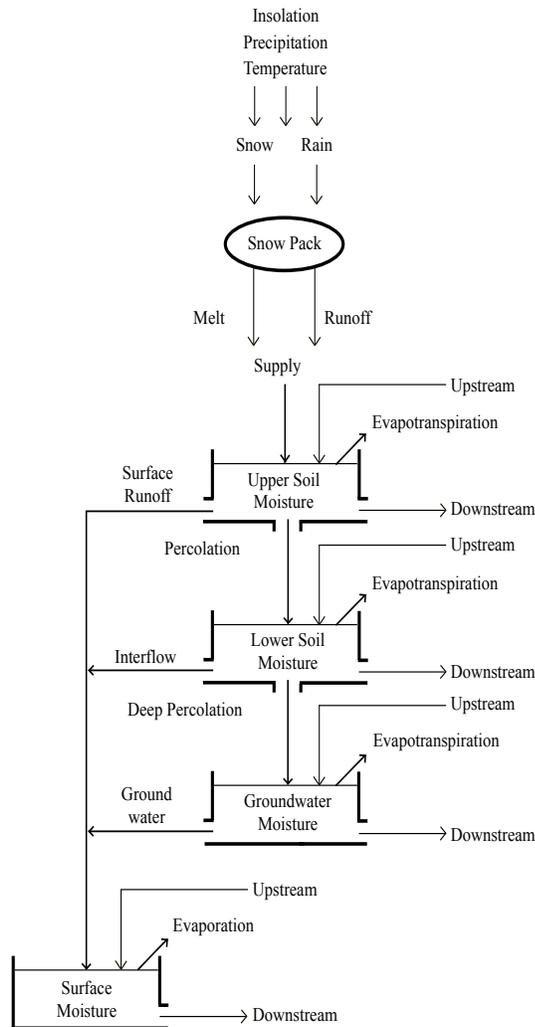
Figure 2. Tank cascade schematic of Distributed Large Basin Runoff Model
