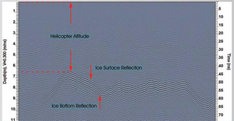
**Figure 3:** Example helicopter-borne GPR data. The data show the ice surface reflection undulating up and down as the helicopter height varies - the GPR acts like a radar altimeter. The goal, however, is to see beneath the surface. The ice bottom reflection is clearly visible.
