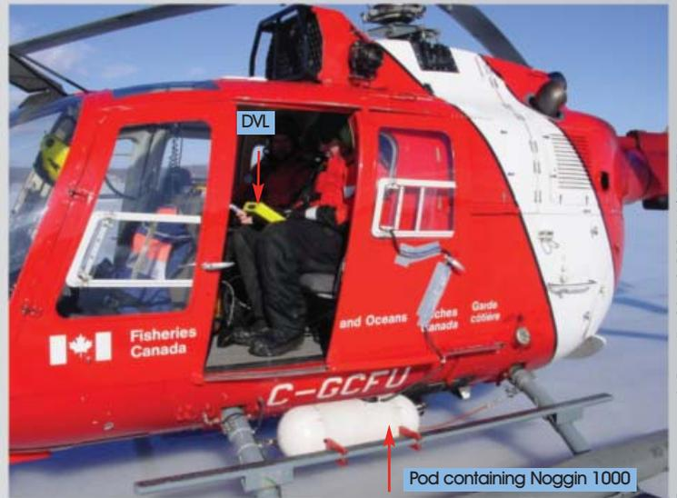
**Figure 2:** A Noggin 1000 is housed in an external pod. The operator observes and records the Noggin data while in flight using a DVL.
