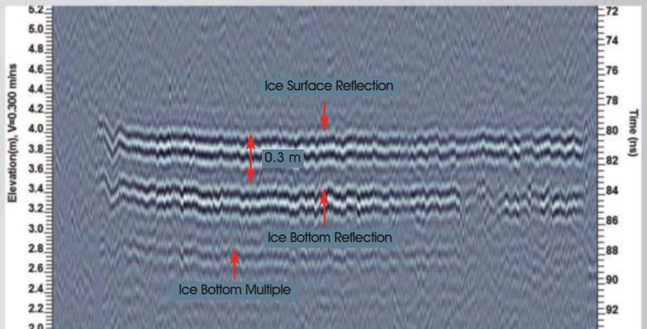
**Figure 4:** Example of data compensated for helicopter height variations.
