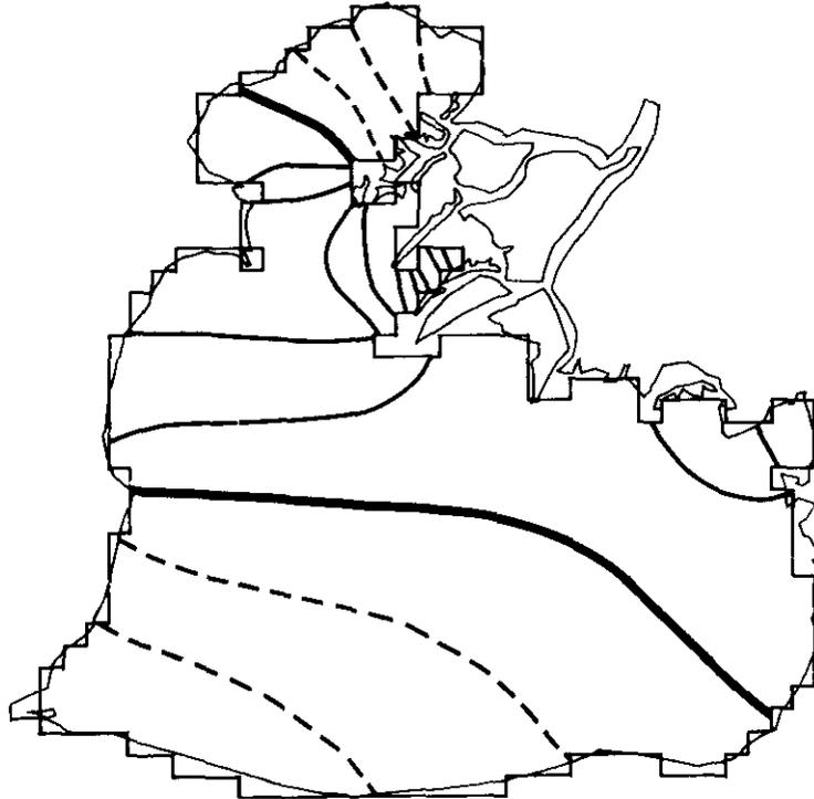
Figure 4.--Amplitude **distribution** for **the third normal mode** of **Lake St. Clair**,
