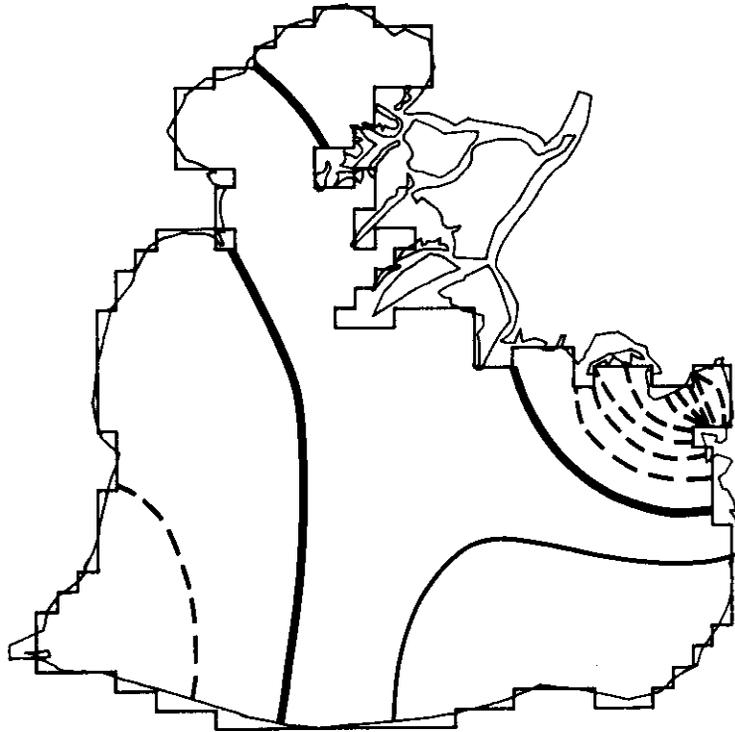
**Figure 5.--Amplitude distribution for the fourth normal mode of Lake St. Clair, with a period of 1.89 h.**
