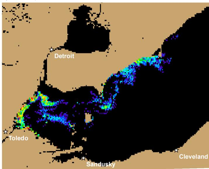
Figure 3. Forecast position of bloom for 11 September 2014 using GLCFS modeled currents to move the bloom from the 7 September 2014 image.
